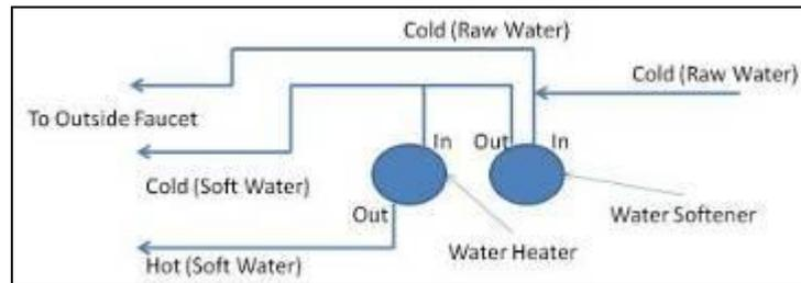
Figure 6. Piping Diagram
