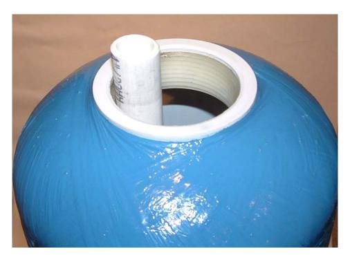
Step 6: Place the funnel into the softener tank as shown below, and slowly pour the resin into the softener tank. Caution: If you purchased a water softener that came with a bag containing gravel, you must add the gravel first before the resin.
